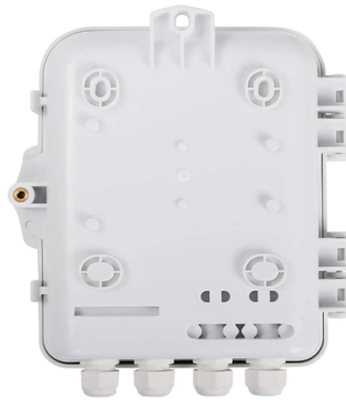
Rear of the optical fiber distribution box
